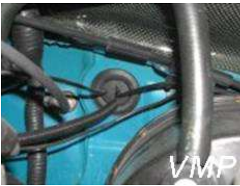
Rubber grommet where blue wire can pass through.(automatic shown)
