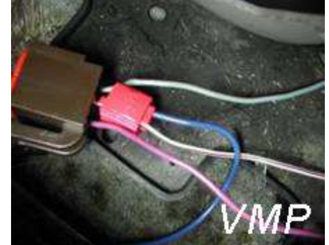
Use pliers and clamp down on metal piece; close wire tap completely.
