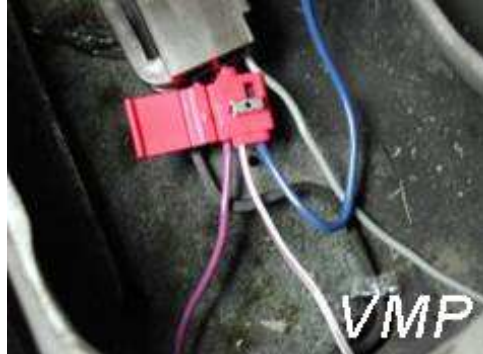
Insert cut pin 2 wire from switch wiring into other hole.
