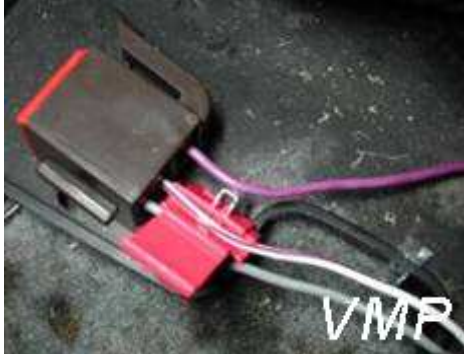
Slide correct wire into wire tap.
