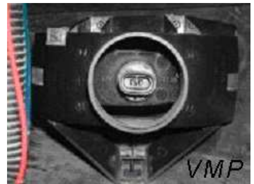
Finished fog light is secure.
