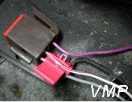
Slide correct wire into wire tap.
