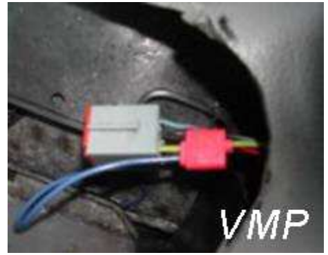
Crimp down metal piece with pliers and close wire tap completely.
