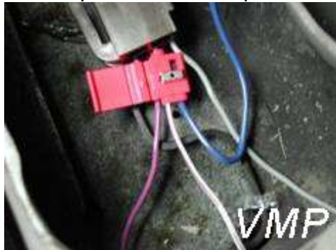
Insert cut pin 4 wire from switch wiring into other hole( Blue wire shown)
