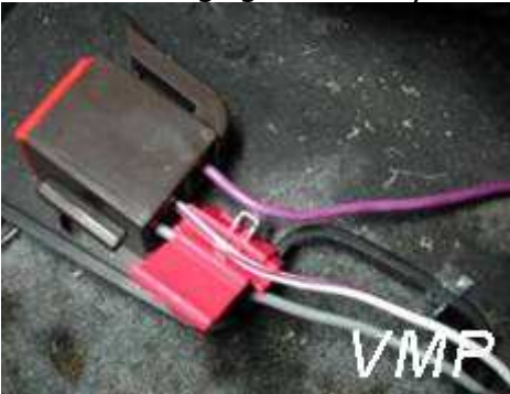
Slide correct wire into wire tap.
