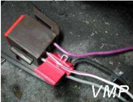
Slide correct wire into wire tap.
